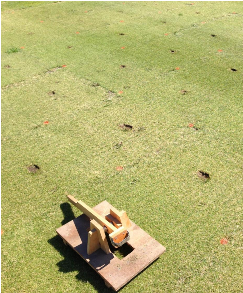
Figure 2. Divots were mechanically removed from each plot with a custom divot-making device. The sheared-off sod was discarded, and the small depression was filled to the soil surface with topdressing sand.
