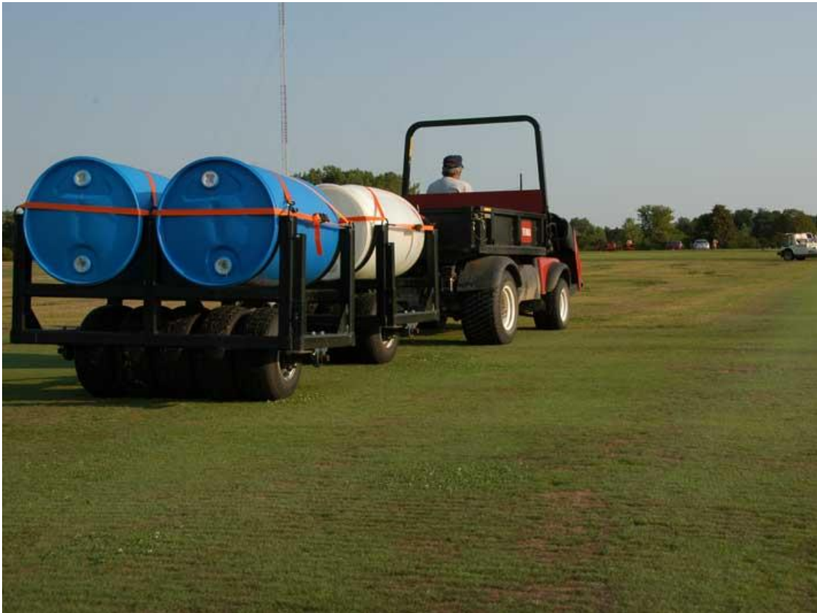
Figure 1. A golf cart traffic simulator weighing roughly 1800 kg was driven across the turfgrass plots. Traffic applications were initiated 1 July and continued to 31 August, for 54 total passes during 2 months of repeated traffic.
